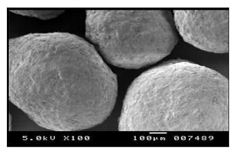
Figure 5: SEM photograph of polymer coated pellets.
