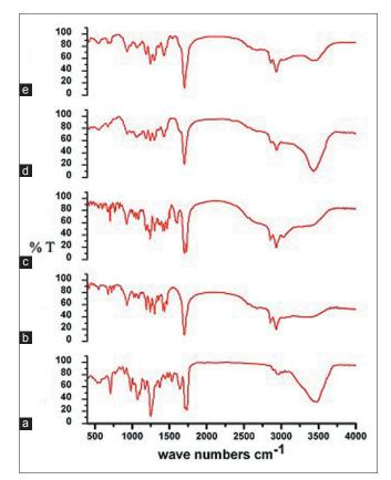
**Figure 2:** Transmission FT-IR spectra of pure PTX (a), pure poly(SA-RA) 70:30 (b), physical mixture of PTX and pure poly(SA-RA) 70:30 (c), F1 (d) and F2 (e)
