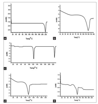
Figure 3: DSC thermograms of pure PTX (a), pure poly(SA-RA) 70:30 (b), physical mixture of drug and polymer (c), F1 (d) and F2 (e)
