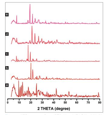
Figure 4: XRD patterns of pure PTX (a), poly(SA-RA) 70:30 (b), physical mixture (c), F1 (d) and F2 (e). The experiment was carried with crimped aluminum pans and a heating rate of 10°C/min; the samples were scanned at 10°C/min from 10 to 230°C
