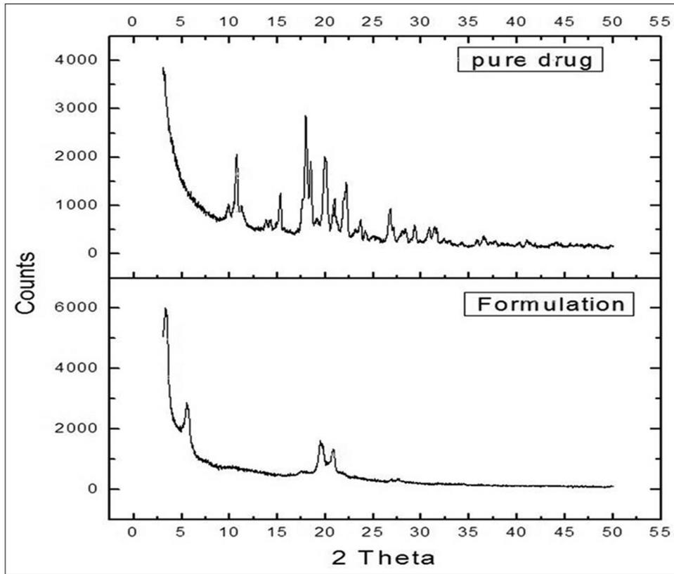
Figure 5: XRD analysis of formulation and pure drug
