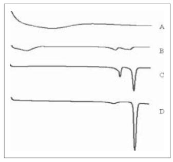
Figure 1: DSC thermogram of A) HPMC, B) solid dispersion, C) physical mixture, and D) CBZ form III
