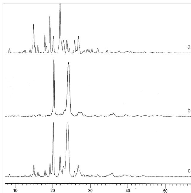
**Figure 1:** XRD patterns of glimepiride (a), poloxamer 188 (b) and solid dispersion (c)
