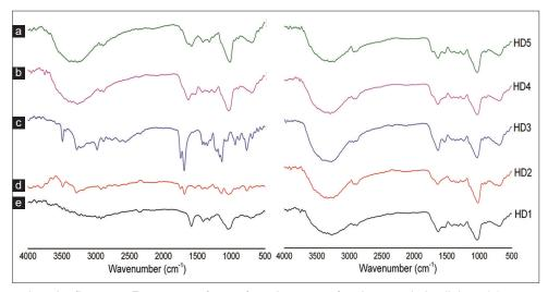
Figure 2: Attenuated total reflectance-Fourier transform infrared spectra of carboxymethyl cellulose (e), tamarind gum (d), citric acid (c), hydrogel dressing (b), and NaOH-treated hydrogel dressing (a) and hydrogel dressings (batch hydrogel dressings HD1-HD5)
