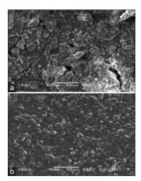
**Figure 5:** Scanning electron microscopy of hydrogel dressing hydrogel dressings (HD1) (a) and HD2 (b)
