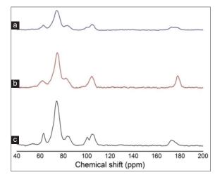
**Figure 4:** Solid-state <sup>13</sup>C-nuclear magnetic resonance of tamarind gum (c), carboxymethyl cellulose (b), and hydrogel dressing (a)
