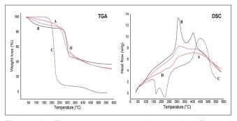
**Figure 3:** Thermogravimetric analysis and differential scanning calorimeter of tamarind gum (a), carboxymethyl cellulose (b), citric acid (c), and hydrogel dressing (d)
