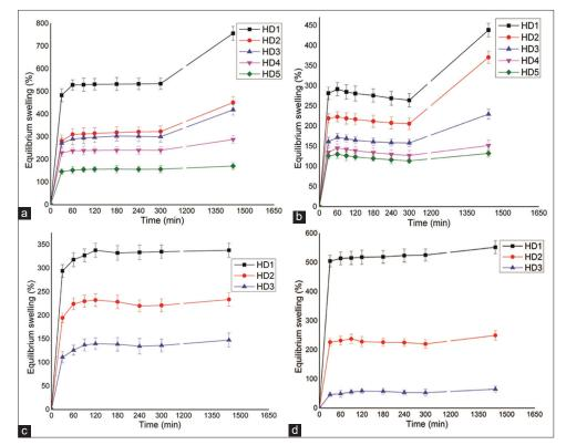
Figure 6: Equilibrium swelling of hydrogel dressing in phosphate buffer (a), 0.1N HCl (b), 0.9% w/v NaCl (c), and water (d)
