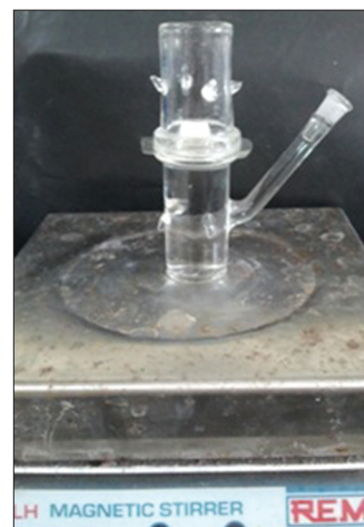
Figure 1: In vitro permeation study using Franz diffusion cell
