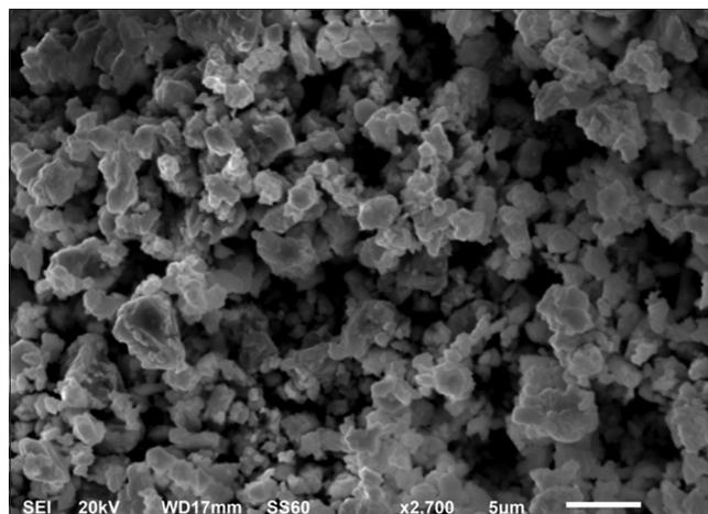
Figure 5: Selenium powder after 4 h grinding scanning electron microscope
