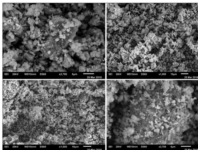
Figure 4: Selenium power after 3 h grinding scanning electron microscope
