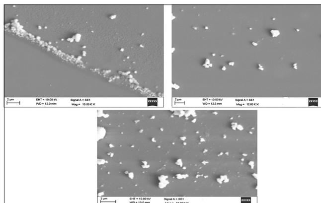
**Figure 7:** SeNPs after ultrasonic irradiation
