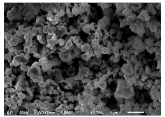
**Figure 5:** Selenium powder after 4 h grinding scanning electron microscope
