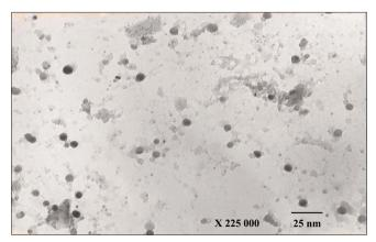
Figure 9: SeNPs after 40 min ultrasonic irradiation transmission electron microscope
