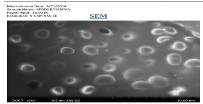
Figure 11: Scanning electron microscope image of self-emulsifying drug delivery system of bosentan FF5 formulation
