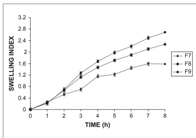
Figure 6: Swelling indices of atenolol from formulations F7, F8 and F9 containing 20, 30 and 40% xanthan gum respectively
