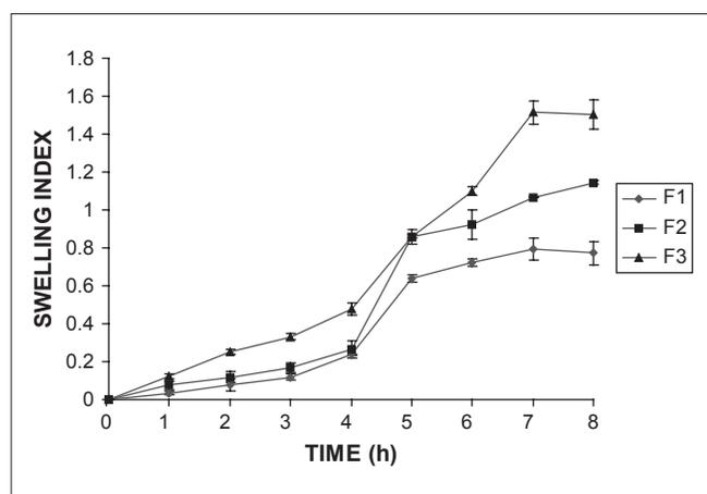
Figure 4: Swelling indices of atenolol from formulations F1, F2 and F3 containing 20, 30 and 40% HPMC K 100 M respectively
