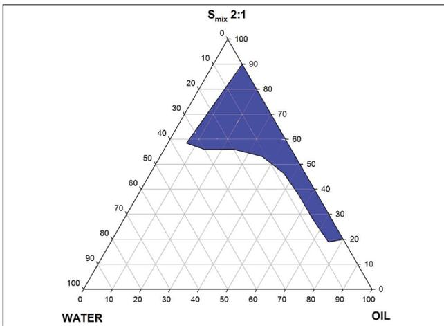
**Figure 3:** Pseudoternary phase diagram for Capryol-90 as oil phase, Acrysol®: TB<sub>3</sub>Mix (2:1) as S<sub>mix</sub> and water
