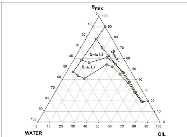
**Figure 5:** Comparative pseudoternary phase diagram for Capryol-90 as oil phase, Acrysol®: TB<sub>3</sub>Mix as S<sub>mix</sub> and water
