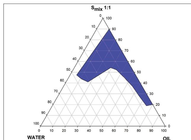
Figure 2: Pseudoternary phase diagram for Capryol-90 as oil phase, Acrysol®: TB<sub>3</sub>Mix (1:1) as S<sub>mix</sub> and water
