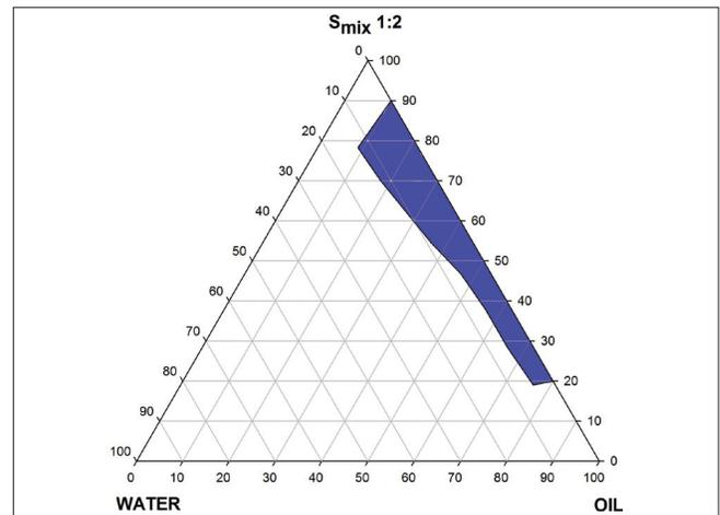
**Figure 4:** Pseudoternary phase diagram for Capryol-90 as oil phase, Acrysol®: TB<sub>3</sub>Mix (1:2) as S<sub>mix</sub> and water
