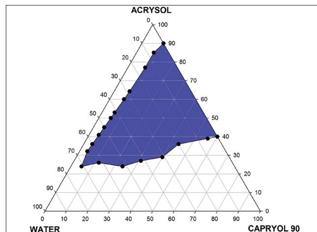
Figure 1: Pseudoternary phase diagram for Capryol-90 as oil phase, Acrysol® as surfactant and water
