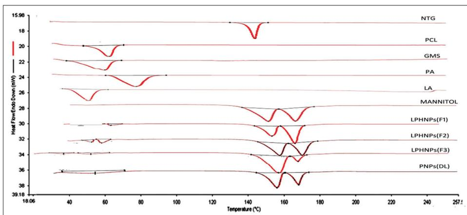
**Figure 3:** DSC thermograms of (A) Nateglinide (NTG), (B) Polycaprolactone (PCL), (C) Glyceryl monostearate (GMS), (D) Palmitic acid (PA), (E) Lauric acid (LA), (F) Mannitol, (G) LPHNPs(F1), (H) LPHNPs(F2), (I) LPHNPs(F3), (J) PNP<sub>s</sub>(DL)
