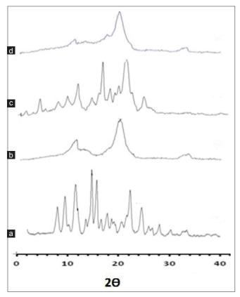
**Figure 1:** X-ray powder diffractograms of carvedilol (a), Avicel pH 101 (b), solid dispersion (SD) formula F6 (c) and surface SD F3 (d)
