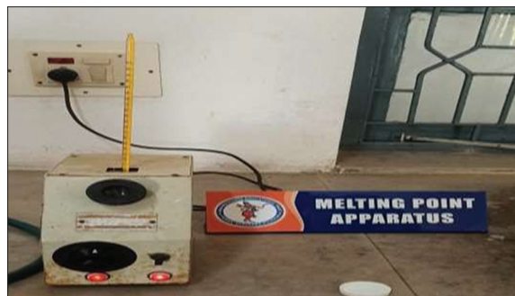
Figure 7: The melting point test performed for the prepared formulation by using the melting point apparatus
