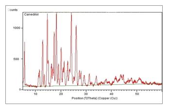
Figure 5: X-ray diffraction of carvedilol
