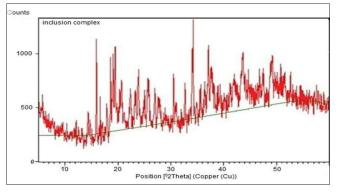
Figure 6: X-ray diffraction of inclusion complex
