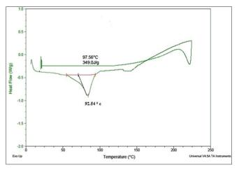
Figure 8: Differential scanning calorimetry thermogram of inclusion complex
