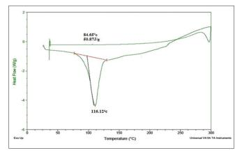
Figure 7: Differential scanning calorimetry thermogram of carvedilol
