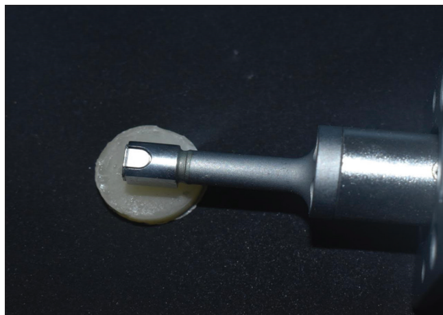
Figure 3: Surface roughness assessment using surface profilometer
