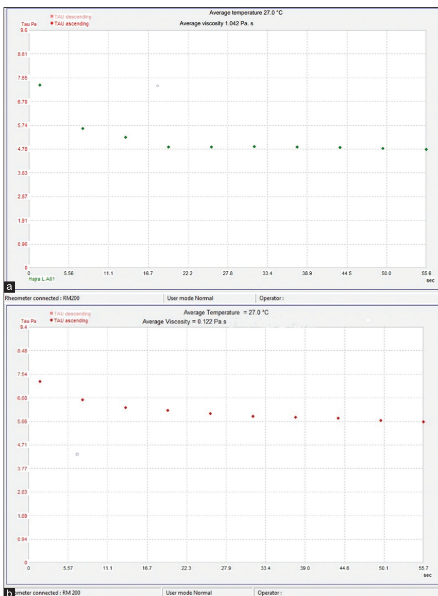
Figure 3: Rheograms of (a) tested emulsion (b) control emulsion
