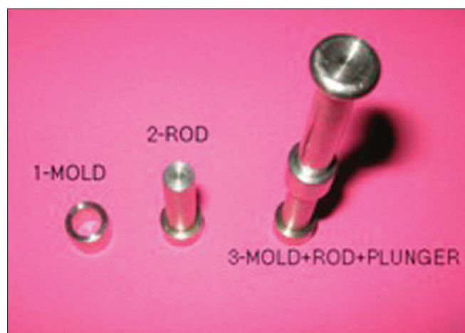
Figure 1: Fabricated a unit, which consists of mold, rod and plunger (melt extrusion)
