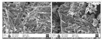
Figure 8: Scanning electron microscopy photographs of pure drug crystals
