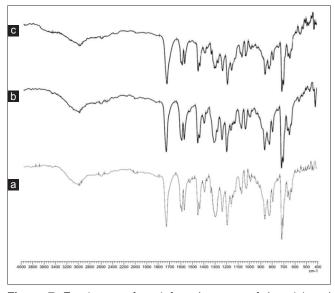
**Figure 7:** Fourier transform-infrared spectra of drug (a) and agglomerates prepared with Eudragit RS100 (b) and Eudragit RL100 (c)
