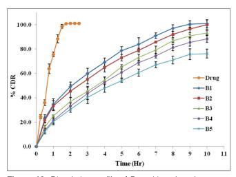
**Figure 12:** Dissolution profile of Drug (•) and agglomerates prepared with Eudragit RL100 (B1 to B5)
