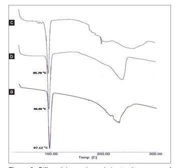
**Figure 6:** Differential scanning calorimetry thermogram of drug (a) and agglomerates prepared with Eudragit RS100 (b) and Eudragit RL100 (c)
