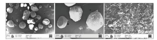
Figure 10: Scanning electron microscopy photographs of agglomerates prepared with Eudragit RL100
