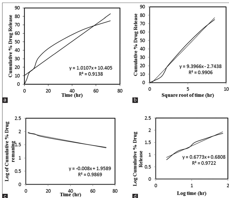
**Figure 8:** Drug release kinetics plots: (a) Zero order plot, (b) Higuchi plot, (c) first order plot and (d) Korsmeyer–Peppas plot
