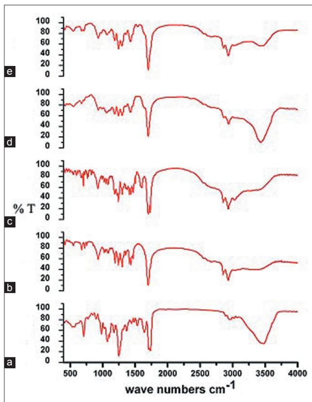
**Figure 2:** Transmission FT-IR spectra of pure PTX (a), pure poly(SA-RA) 70:30 (b), physical mixture of PTX and pure poly(SA-RA) 70:30 (c), F1 (d) and F2 (e)
