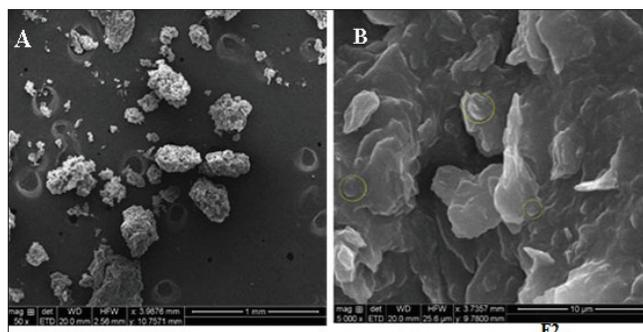
**Figure 1:** Typical scanning electron micrographs of poly(SA-RA) 70:30nanoparticles: (A) blank NPs and (B) PTX loaded NPs (F2)
