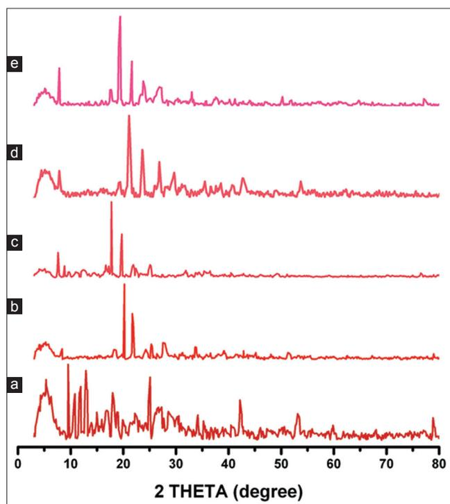
Figure 4: XRD patterns of pure PTX (a), poly(SA-RA) 70:30 (b), physical mixture (c), F1 (d) and F2 (e). The experiment was carried with crimped aluminum pans and a heating rate of 10°C/min; the samples were scanned at 10°C/min from 10 to 230°C
