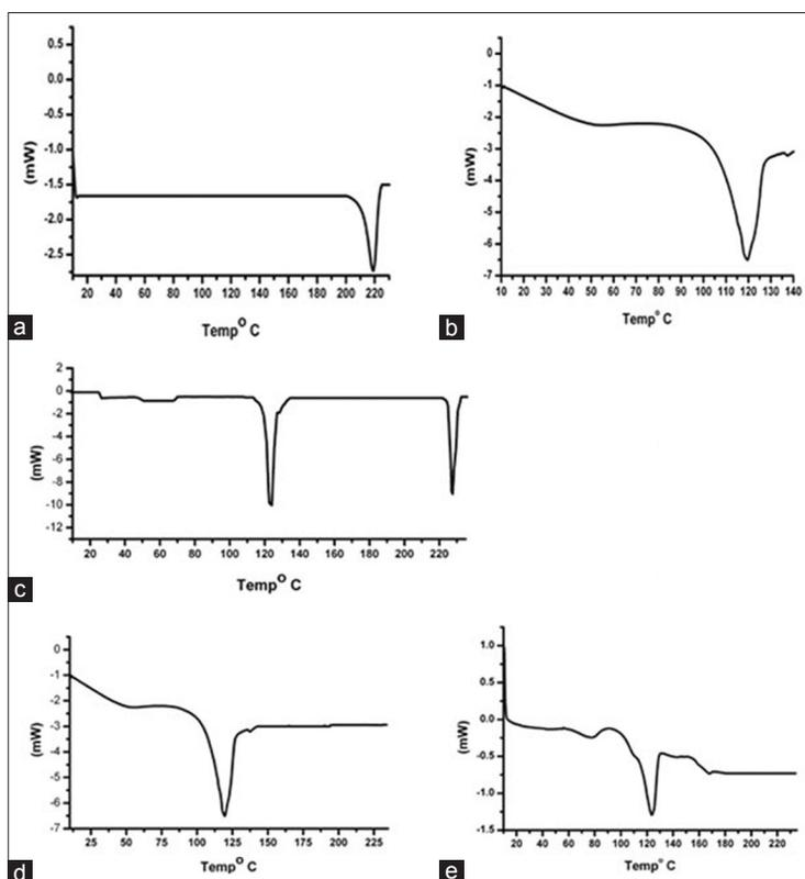
Figure 3: DSC thermograms of pure PTX (a), pure poly(SA-RA) 70:30 (b), physical mixture of drug and polymer (c), F1 (d) and F2 (e)
