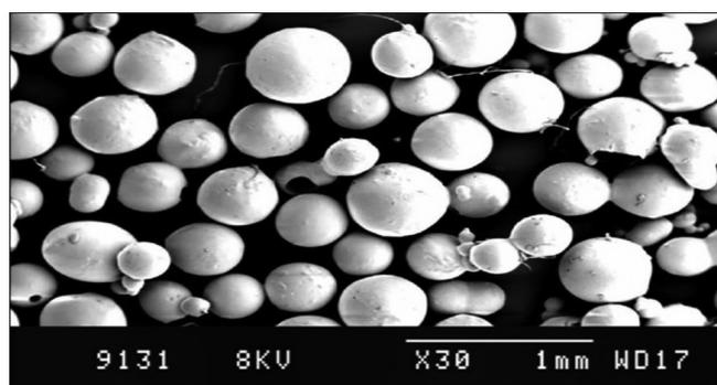
**Figure 1:** SEM photomicrograph of alginate microspheres without drug
