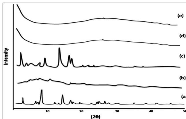
**Figure 4:** XRD of (a) DF, (b) alginate, (c) mixture of DF and alginate, (d) alginate microspheres without drug, (e) alginate microspheres loaded with drug
