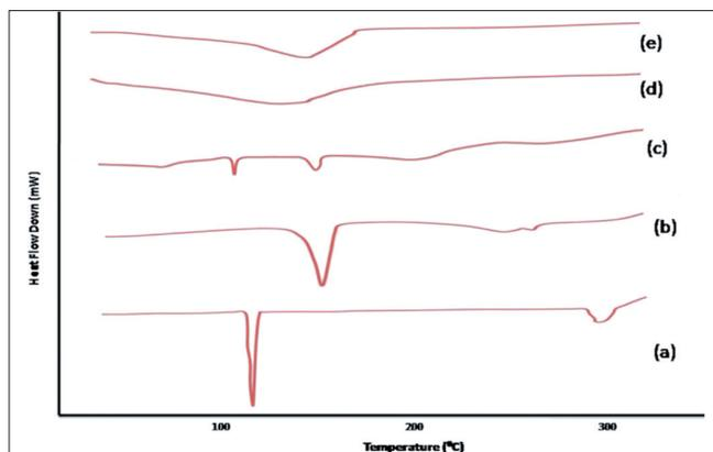
**Figure 3:** DSC thermogram of (a) diloxanide furoate (DF; Drug) (b) alginate (Polymer) (c) mixture of DF and alginate (d) alginate microspheres without drug (e) alginate microspheres loaded with drug
