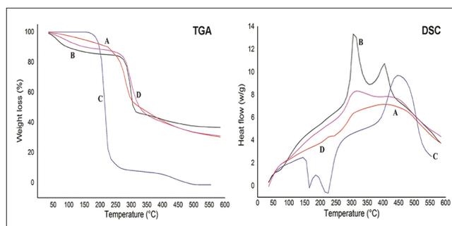
**Figure 3:** Thermogravimetric analysis and differential scanning calorimeter of tamarind gum (a), carboxymethyl cellulose (b), citric acid (c), and hydrogel dressing (d)
