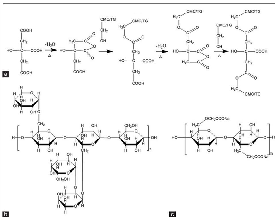
**Figure 1:** Possible cross-linking reaction between citric acid, tamarind gum (TG), and carboxymethylcellulose (CMC) (a) and structure of TG (b) and CMC (c)
