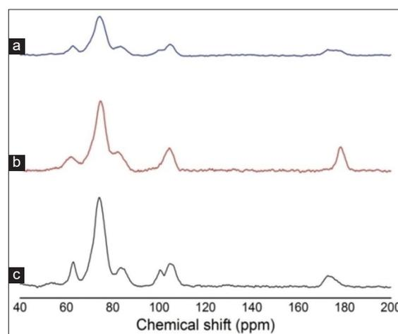
**Figure 4:** Solid-state  $^{13}\text{C}$ -nuclear magnetic resonance of tamarind gum (c), carboxymethyl cellulose (b), and hydrogel dressing (a)
