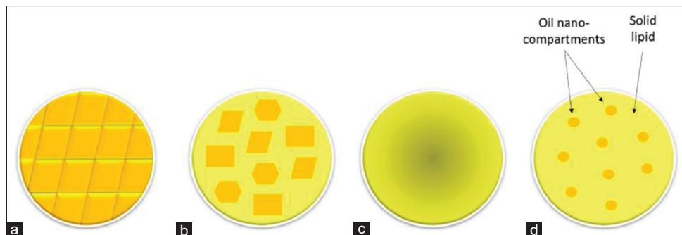
**Figure 4:** Schematic representation of solid lipid nanoparticles and different nanostructured lipid carrier (NLC type). (a) Solid lipid nanoparticles; (b) imperfect nanostructured lipid carrier; (c) structure less nanostructured lipid carrier; (d) multiple oil in solid fat in water<sup>[12]</sup>
