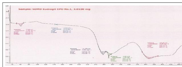
**Figure 2:** Differential scanning calorimetry thermogram of Doxazosin - Eudragit EPO spray dried microspheres
