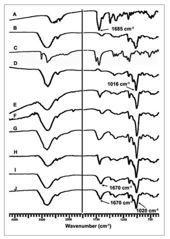
**Figure 4:** Infrared spectra of pure domperidone (DOM) (A),  $\beta$ -cyclodextrin ( $\beta$ CD) (B), citric acid (CA) (C), mannitol (D), physical mixtures of DOM/ $\beta$ CD (E), DOM/ $\beta$ CD/CA (F), DOM/  $\beta$ CD/CA/mannitol (G) and kneaded complexes of DOM/  $\beta$ CD (H), DOM/ $\beta$ CD/CA (I), and DOM/ $\beta$ CD/CA/mannitol (J)
