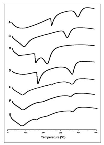
**Figure 5:** Differential scanning calorimetry thermograms of domperidone (DOM) (A),  $\beta$ -cyclodextrin ( $\beta$ CD) (B), citric acid (CA) (C), mannitol (D), and kneaded complexes of DOM/ $\beta$ CD (E), DOM/ $\beta$ CD/CA (F), and DOM/ $\beta$ CD/CA/mannitol (G)
