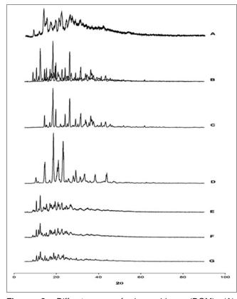
**Figure 6:** Diffractogram of domperidone (DOM) (A),  $\beta$ -cyclodextrin ( $\beta$ CD) (B), citric acid (CA) (C), mannitol (D), and kneaded complexes of DOM/ $\beta$ CD (E), DOM/ $\beta$ CD/CA (F), and DOM/ $\beta$ CD/CA/mannitol (G)
