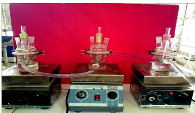
**Figure 12:** Diffusion cell Assembly used in experimental work for drug release study
