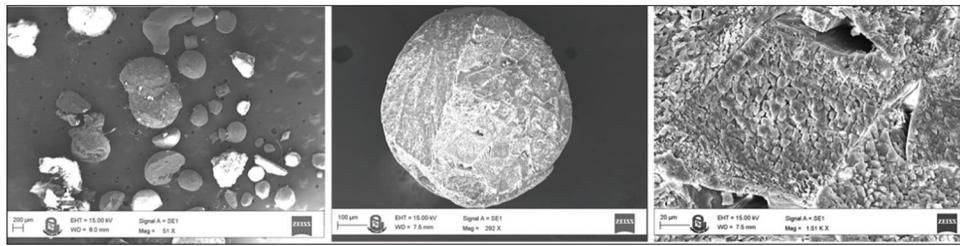
Figure 9: Scanning electron microscopy photographs of agglomerates prepared with Eudragit RS100
