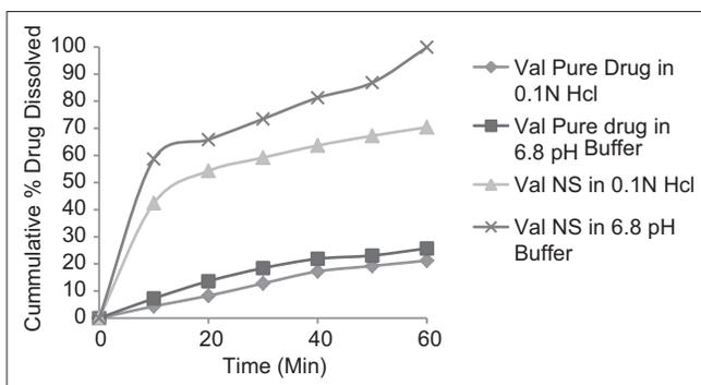
**Figure 10:** Dissolution profile Valsartan pure drug and optimized nanosuspension in 0.1N HCl and 6.8 pH phosphate buffer
