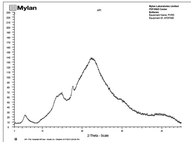
Figure 5: Powder X-ray diffraction pattern of pure drug (Valsartan)
