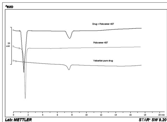
**Figure 3:** Differential scanning calorimetry thermogram of pure drug, poloxamer and nanosuspension
