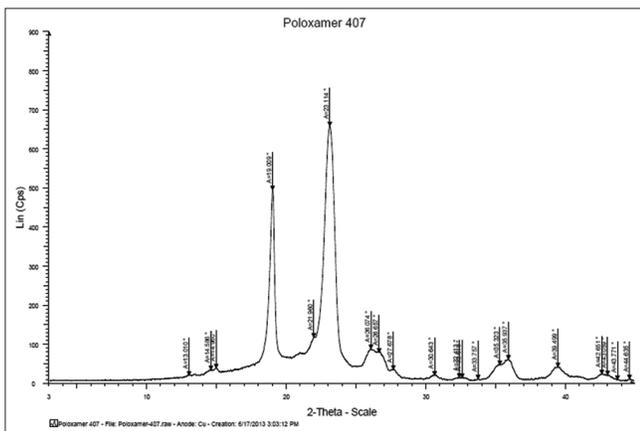
Figure 6: Powder X-ray diffraction pattern of poloxamer
