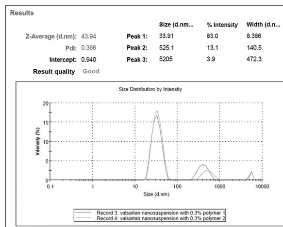
**Figure 2:** Particle size distribution by Malvern particle size analyzer
