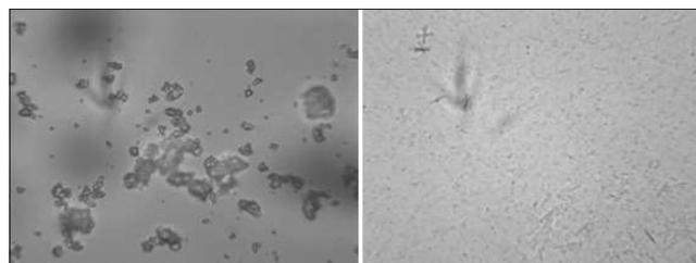
**Figure 1:** Optical microscopic image of Valsartan suspension and nanosuspension at X40
