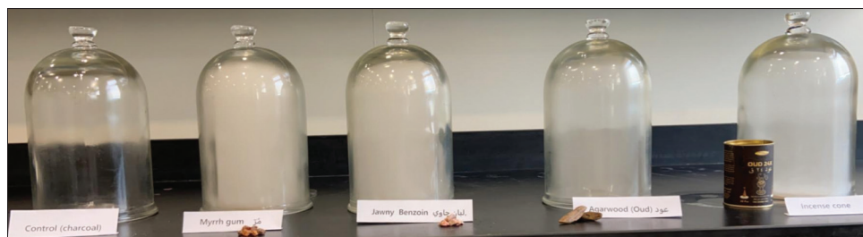
Figure 2: Resin fumes and experimental setup of bell jar exposure study
