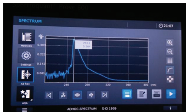
Figure 2: Ultraviolet spectrometric analysis of Peppermint essential oil
