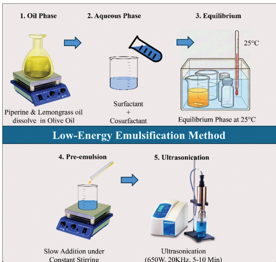
Figure 1: Schematic representation of the low-energy ultrasonication method for nanoemulsion preparation
